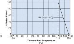
For resistors operated terminal temperature of described for each size or above, a power rating shall be derated in accordance with the derating curve.
